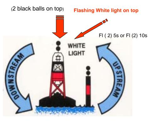
Isolated danger underneath buoy
