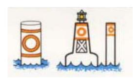
**Control Buoy:** Usually with speed limit or no wash restriction signage
