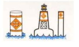
**Keep Out Buoy:** Denies access to buoyed off area often with a heavy fine attached e.g. end of runway for Toronto Island Airport
